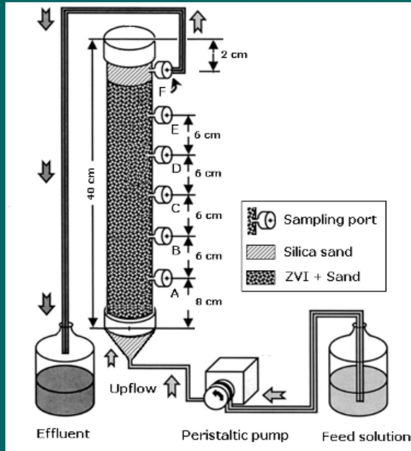
Column system used for pretreatment of oil mill wastes
