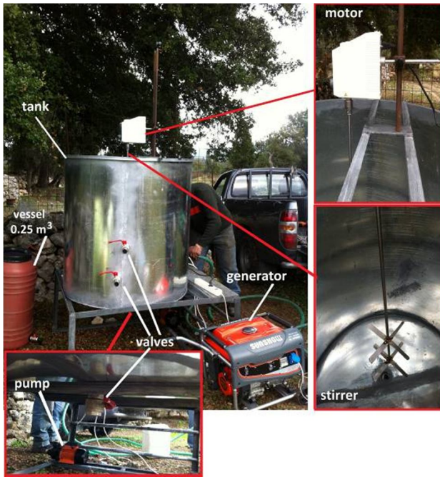
Photo 1. Equipment and accessories for the implementation of OMW pre-treatment in the field
