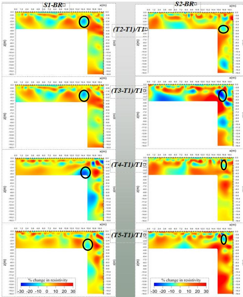
Figure 5: Results of the difference inversion of the ERT data collected along lines S1-BR and S2-BR for the five time phases. The results are plotted in terms of percentage relative change of the model resistivity of each phase with respect to the reference phase. The black circles indicate an area of reduced resistivity that could be attributed to the downwards movement of the OOMW.
