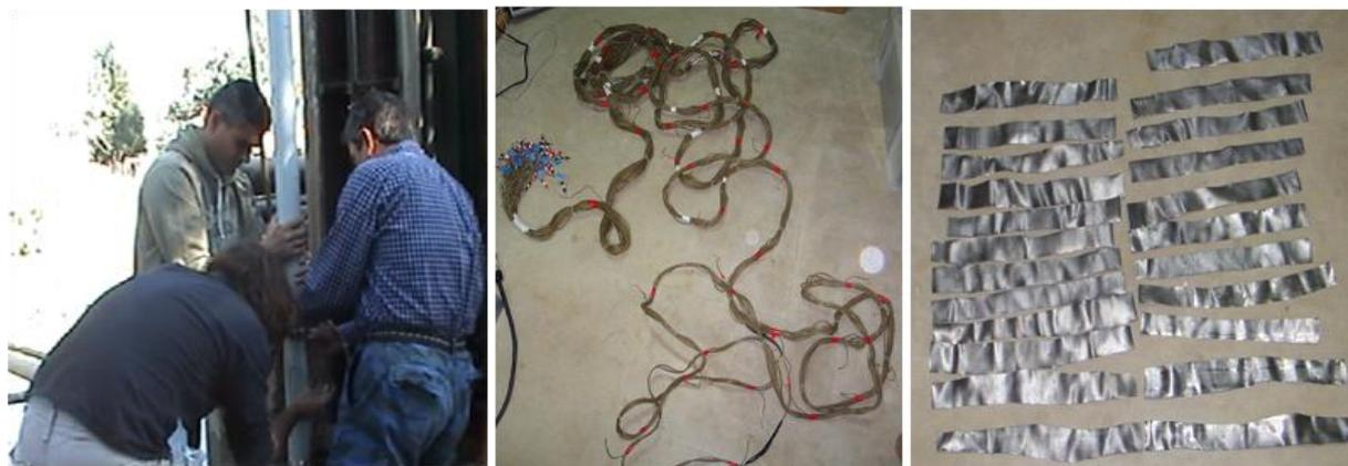
*Figure 2: (left) Installation of the multi-node cable on the outer surface of the plastic piezometer that was placed inside the borehole. Custom made multi-node cable with 48 electrode outputs (middle) and lead leaves that were used as borehole electrodes (right).*
