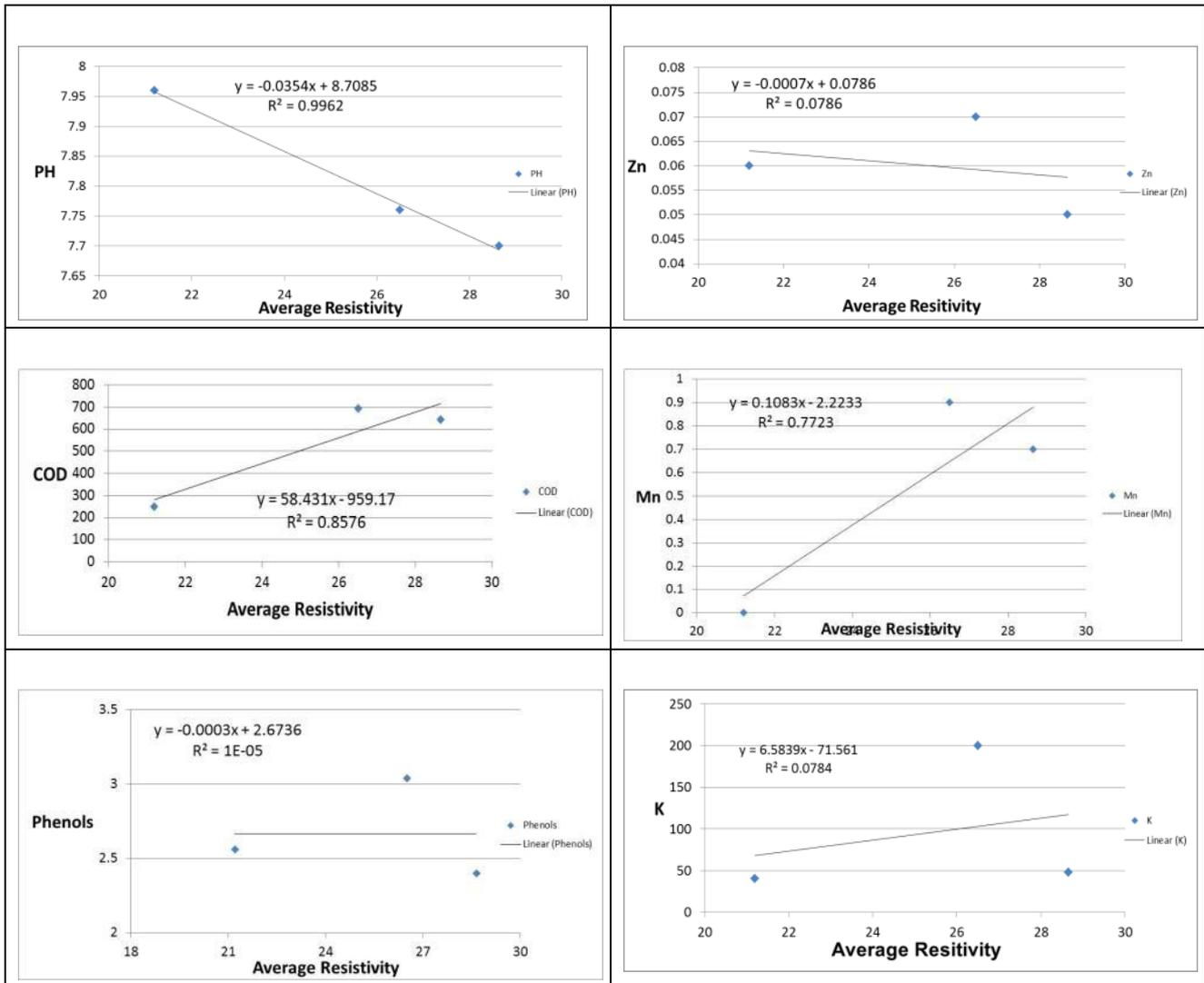
Figure 6: Correlation function between the inverted bulk resistivity (from ERT measurements) and measurements of various chemical elements.
